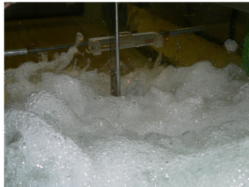
(C) Fr_1 = 7.5 , Re = 5.6 \times 10^4 , d_1 = 0.018 m, x_1 = 0.75 m, shutter speed: 1/80 s - From Top Left, anti-clockwise: (C1) Side view with the probe tip located at x-x_1 = 0.075 m; (C2) Looking upstream above the roller with the probe tip located at x-x_1 = 0.075 m; (C3) Looking upstream above the roller with the probe tip located at x-x_1 = 0.35 m; (C4) Looking downstream at the jump toe with the probe tip located at x-x_1 = 0.35 m
