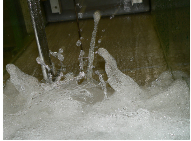
(A) Looking downstream at the jump toe with the probe tip located at x-x_1 = 0.075 m - Fr_1 = 5.1 , Re = 4.0 \times 10^4 , d_1 = 0.0185 m, x_1 = 0.75 m, shutter speed: 1/80 s
