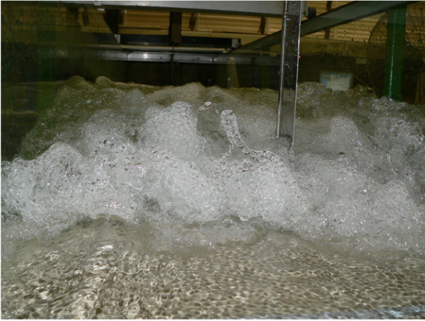
(A) Looking downstream at the jump toe with the probe tip located at x-x_1 = 0.075 m - Fr_1 = 5.1 , Re = 4.0 \times 10^4 , d_1 = 0.0185 m, x_1 = 0.75 m, shutter speed: 1/80 s
