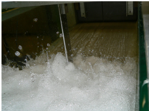
(C) Fr_1 = 7.5 , Re = 5.6 \times 10^4 , d_1 = 0.018 m, x_1 = 0.75 m, shutter speed: 1/80 s - From Top Left, anti-clockwise: (C1) Side view with the probe tip located at x-x_1 = 0.075 m; (C2) Looking upstream above the roller with the probe tip located at x-x_1 = 0.075 m; (C3) Looking upstream above the roller with the probe tip located at x-x_1 = 0.35 m; (C4) Looking downstream at the jump toe with the probe tip located at x-x_1 = 0.35 m
