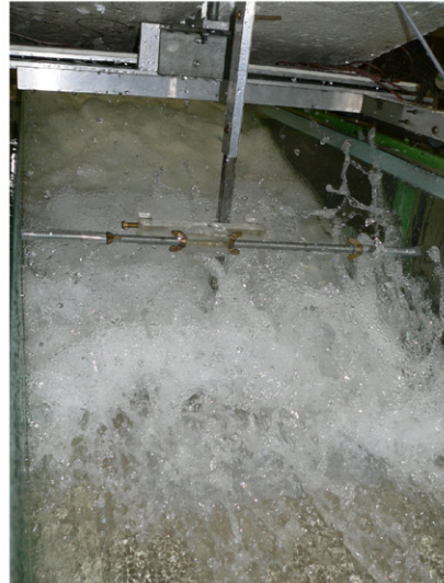
(A) Looking downstream at the jump toe with the probe tip located at x-x_1 = 0.075 m - Fr_1 = 5.1 , Re = 4.0 \times 10^4 , d_1 = 0.0185 m, x_1 = 0.75 m, shutter speed: 1/80 s
